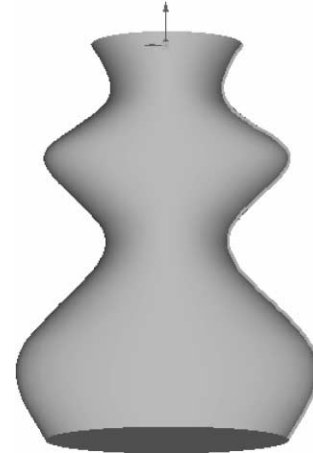
Fig. 7. Single-direction symmetric deformation rule.
